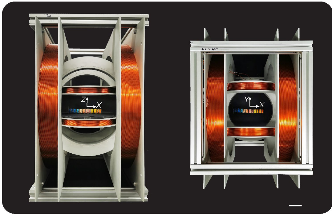
Fig. S4. Front view and top view of the 3D Helmholtz coils with a 12-unit octopus-like robotic arm inside the magnetic apparatus. Scale bar: 5 cm.
