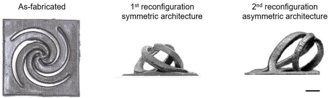
Figure S21. 2D-to-3D and 3D-to-3D structural reconfigurations of MDP. Scale bar: 5 mm.
